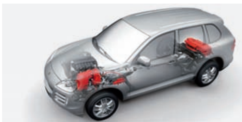
When developing a concept for the planned Cayenne Hybrid, Porsche engineers in Weissach opted for a parallel full hybrid system.
